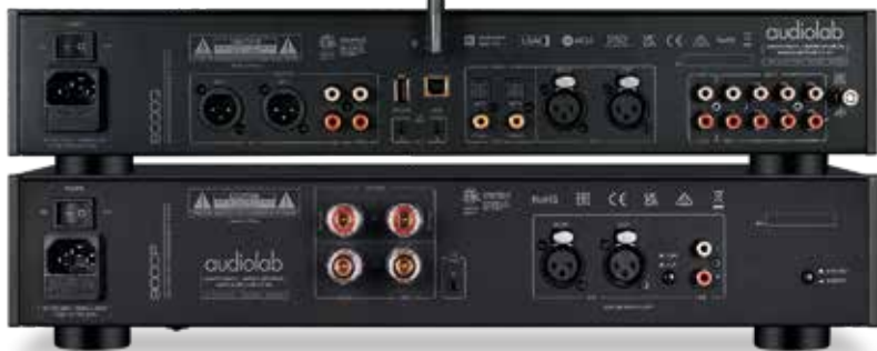
ABOVE: 9000Q [top] has MM and four line ins (one balanced on XLR), a line out and three pre outs (two on RCA, one balanced XLR). Digital ins include coax/opt digital (192kHz/24-bit) and USB-B (768kHz/DSD512). 9000P [bottom] has RCA and balanced XLR ins and outputs on 4mm binding posts. Note bridging option [see boxout, p63]
