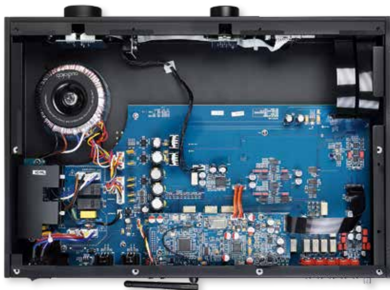
ABOVE: Linear PSU [left] feeds regulated supplies for the digital board [bottom] with its Feasycom BT audio module, XMOS USB receiver and tried-and-tested ESS ES9038PRO DAC. Analogue preamp PCB includes MM phono stage [bottom right]
